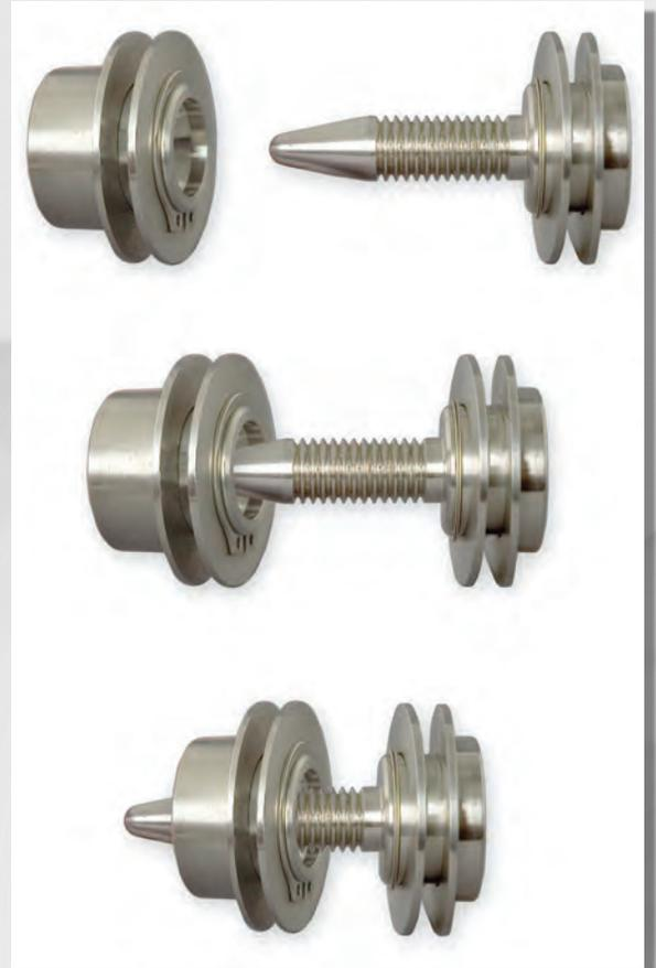
**Notice the conical tip on the male component to help alignment for smooth fastening into the female component. To prevent loosening due to vibration or rotation, radial grooves in the components replace the helical threads normally used in fasteners. Once the ZipNut fasteners engage, the action is irreversible.**
